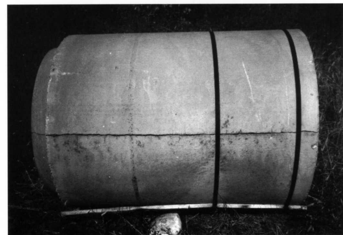
The 30 inch test pipes were temporarily banded and broken into 4 quadrants. Then all pipe sections were placed in the soil cell with only the backfill supporting them.
