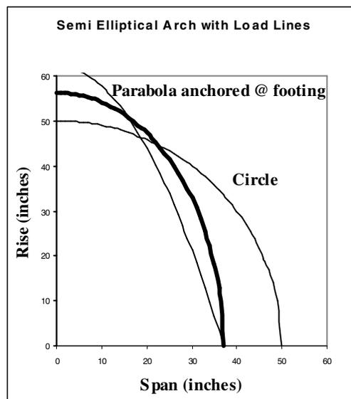
**Figure 2.** Semi elliptical arch and two funicular load curves.
