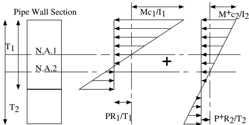
**Figure 3.** General wall stress in deteriorated wall ( $T_1$ ) and rehabilitated wall ( $T_2$ ).
