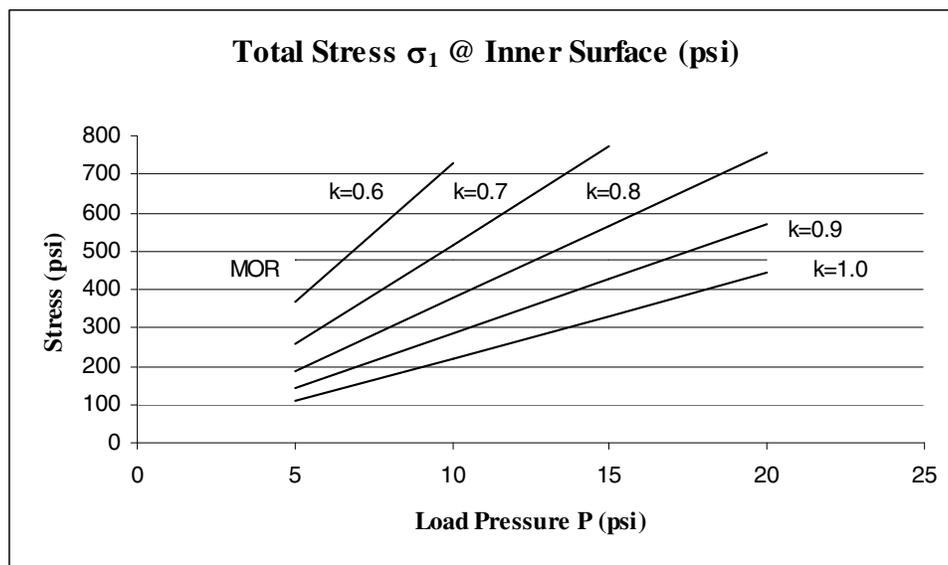
**Figure 4.** Stress levels for  $R_0 = 46''$ ,  $T_0 = 7.5''$  and  $K' = 0.75$ .
