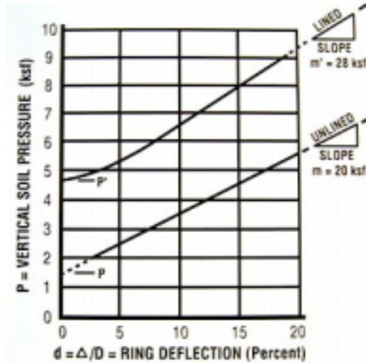
**Figure 3. Utah Load-deflection Data for Lined and Unlined Pipes**
